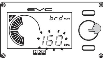
(2) Turn volume knob and select the max value to be displayed on the bar graph. When selection is done, press the volume knob again.
