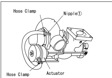
(1) Remove the hose which connects the actuator and Nipple 1 from the compressor side.
