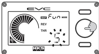
(2) Turn the volume knob to select input signal function. After selection, press the volume knob.
