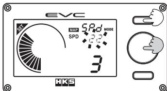
(3) Turn the volume knob and change the speed corresponding to the grid point. When the setting is done, press the volume knob again.
