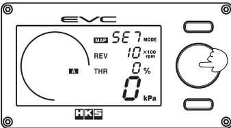
(1) Press the volume knob in the boost map correction A set mode or B set mode.
