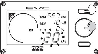
(2) Turn the volume knob to set the correction boost. When settings are complete, press the volume knob again.
