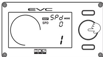
(1) Press the volume knob while in the speed axis grid point set mode.
