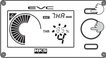
(3) Turn the volume knob and change the throttle opening % corresponding to the grid point. When the setting is done, press the volume knob again.
