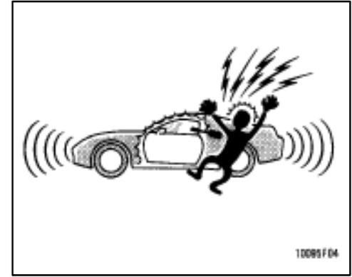
To deter the vehicle theft, the system is designed to give an alarm and keep the engine from being started if any of the side doors, back door or hood is forcibly unlocked or the battery terminal is disconnected and then reconnected when the vehicle is locked.
