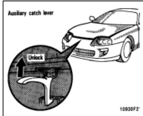
2. In front of the vehicle, pull up on the auxiliary catch lever and lift the hood.
