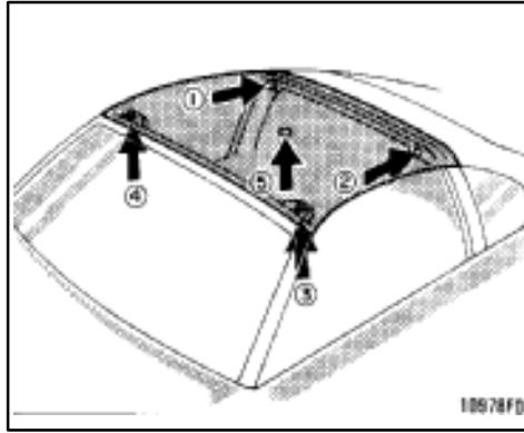
**3. Tighten the bolts and lock the center lock in the order shown. (See “–Detaching from vehicle” for details.)**
