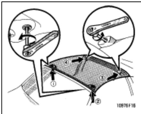
4. Loosen the bolts in the order shown by turning the wrench counterclockwise. Then lift up the front edge of the sport roof and lift off the roof forward.
