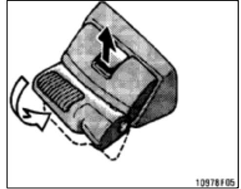
After removing the roof, put back the rear holders by pulling up the lock release knob.
