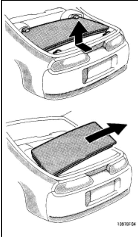
1. Lift up the rear edge while pushing the roof fully forward, then pull the front edge out of the holders. Remove the roof from the right side as shown.
