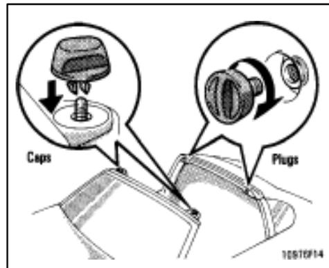
5. After removing the roof, put the caps on the front bolts and insert the plugs into the rear holes
