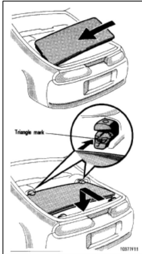
2. Put in the roof from the left side as shown. Then insert the front edge of the roof in the front holders, and engage the rear edge with the rear holders.
