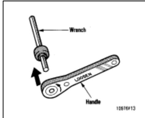
**2. Face the “LOOSEN” side of the handle toward you and insert the wrench into the handle.**
