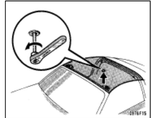
**3. Unlock the center lock by inserting the wrench and turning it a 1/4 turn counterclockwise.**
