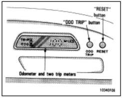
This meter displays the odometer and two trip meters. To change the odometer display to the trip meter display, push the "ODO TRIP" button. To reset the trip meter A to zero, display the meter A reading, then push the "RESET" button. The same applies for the trip meter B.
