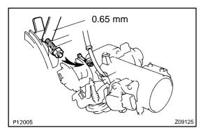
(b) Insert a 0.65 mm (0.026 in.) feeler gauge between the throttle stop screw and stop lever.
