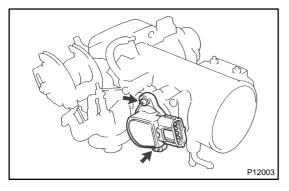
(c) Using an ohmmeter, measure the resistance between terminals.
