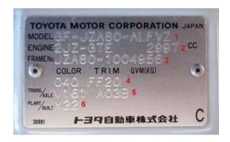
VIN-Plate of a J-Spec vehicle (EU-Spec vehicles do have a slightly different plate)
