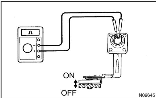
**15. INSPECT ENGINE OIL LEVEL WARNING SWITCH CONTINUITY**
