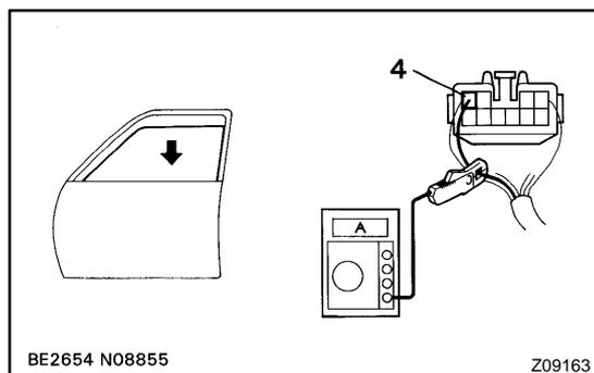
**4. Using an ammeter with a current-measuring probe:
