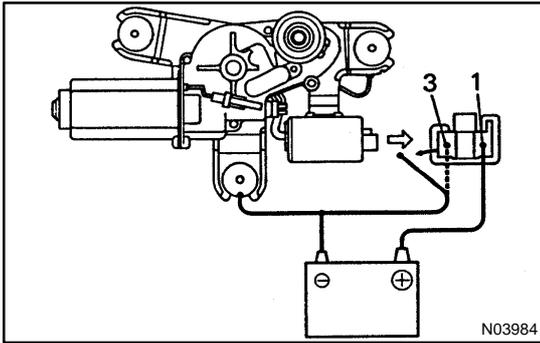
(b) Disconnect the negative (-) lead from terminal 3, check that the motor stops running at the stop position. If operation is not as specified, replace the motor and relay.
