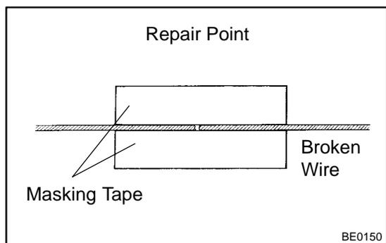
5. IF NECESSARY, REPAIR DEFOGGER WIRE
