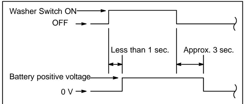
If operation is not as specified, replace the wiper and washer switch.
