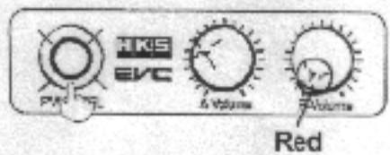
(9) Press the (PWR/SEL) button once (short press) and verify that the ▲ on volume knob B is lit up red.
