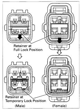
Push the terminal retainer down to the temporary lock position.
