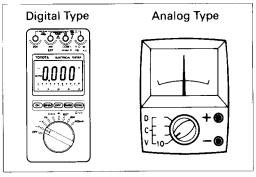
(c) Use the volt/ohmmeter with high impedance (10 kΩ/V minimum) for troubleshooting of the electrical circuit.
