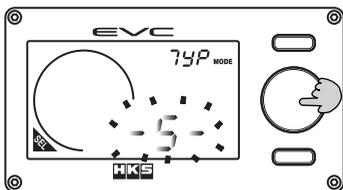
(1) Turn the volume knob and select the exhaust bypass type from "-S-" for the swing valve type or "-P-" for the poppet valve type.
