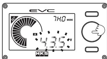
(2) The current throttle voltage is displayed. When the **A** icon is illuminated, the voltage will be automatically determined. With the engine OFF, firmly step on the accelerator pedal until it reaches the stopper. After confirming that it is fully open, press the volume knob to set the value.
