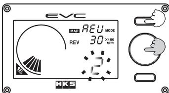
(2) Turn the volume knob to select the grid point to change. Press Button ① to change the RPM.
