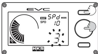
(2) Turn the volume knob to select the grid point to change. Press the Button ① to change the speed value.
