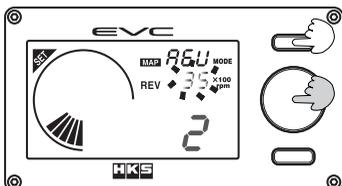
(3) Turn the volume knob and change the RPM corresponding to the grid point. When the setting is done, press the volume knob again.
