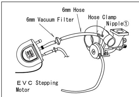
(2) Connect Nipple 1 and the EVC Stepping Motor's 6mm vacuum filter using the included 6mm hose.
