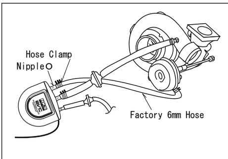
(3) Connect the factory hose, which is still connected to the actuator, to the EVC Stepping Motor's Nipple O.
