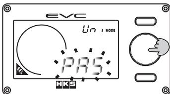
(1) Turn the volume knob and select the pressure unit of measure from "PAS (kPa)" or "PSI."
