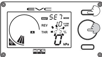
(3) Turn the volume knob to move the throttle opening axis. Pressing Button ① will move to the RPM Axis
