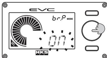
(2) Turn the volume knob to set the function ON or OFF. When the selection has been made, press the volume knob.
