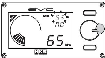
(1) Turn the volume knob and set the max baseline / default boost value if the boost value is known. If not, drive the vehicle under load to achieve the maximum boost value. The value will then be shown in the digital display (S).
