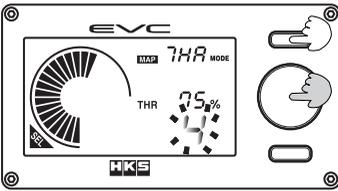
(2) Turn the volume knob to select the grid point to change. Press Button ① to change the throttle opening ratio.
