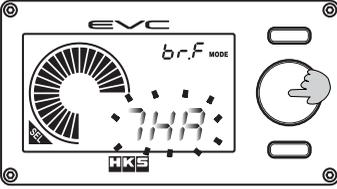
(2) Turn the volume knob to select the data function to be displayed. Press volume knob to complete setting.
