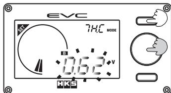
(3) The throttle-off voltage value can also be manually inputted. Press Button ① and the **B** icon will now illuminate, indicating you are in manual mode. Turn the volume knob to select the closed voltage and press the volume knob to set.
