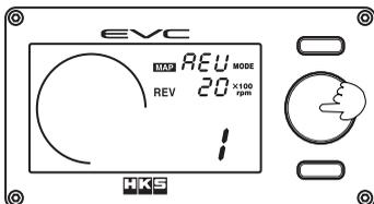
(1) Press the volume knob while in the RPM axis grid point set mode.
