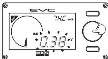
(2) The current throttle voltage is displayed. When the **A** icon is illuminated, the voltage will be automatically determined. To ensure that the throttle is completely closed, step on the accelerator pedal and then release. After confirming that it is closed, press the volume knob to set the value.
