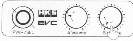
(10) Lightly press volume knob B to pop-up the knob. Turn the knob full counter-clockwise.
