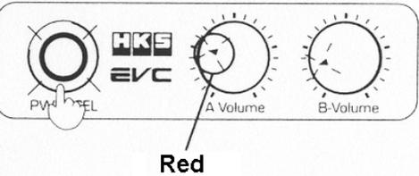
(13) Press the (PWR/SEL) button to enable the boost setting for Mode A, otherwise the boost setting for Mode B will be activated.
