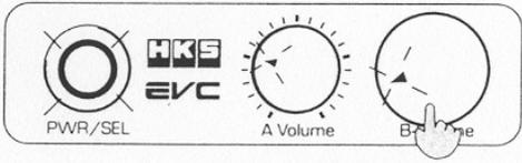
(11) Like the setup for Mode A, repeat steps (4) ~ (6) until the target boost is obtained.
