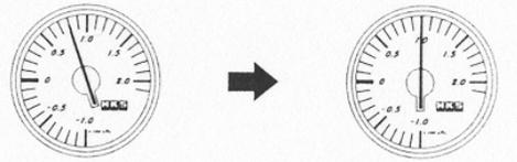
(12) When the projected boost level is reached, press volume knob B back into the unit.
