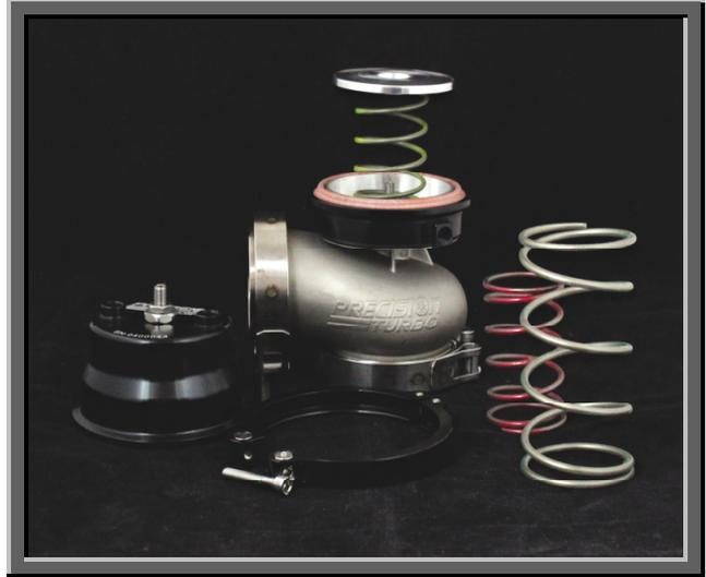
4. Orient the wastegate can top to the desired position and compress the wastegate can top until it is seated with the wastegate can bottom. Use of a press or vice may be necessary depending on spring selection. With the v-band flanges properly aligned, install the v-band clamp. If you need to re-align the upper can, relieve tension on top, rotate and recompress. Once aligned properly, tighten the clamp screw to 51-55 inch lbs or 5 ft lbs. (5.8 – 6.2 Newton Meters)
