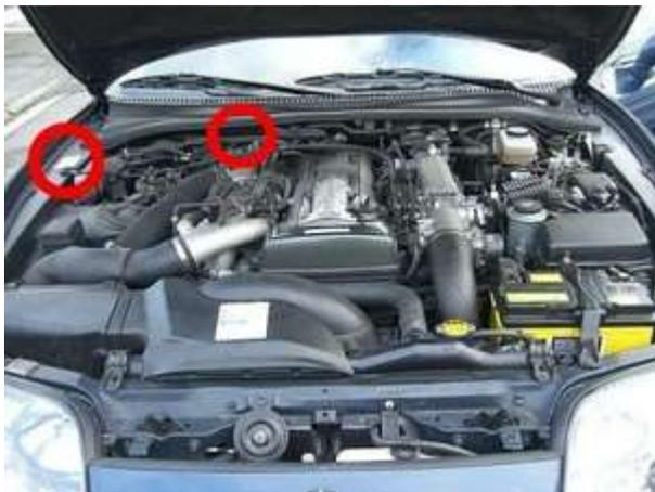
Position of the VIN-Plate (left circle) and the VIN-Number engraved in the firewall (right circle)
