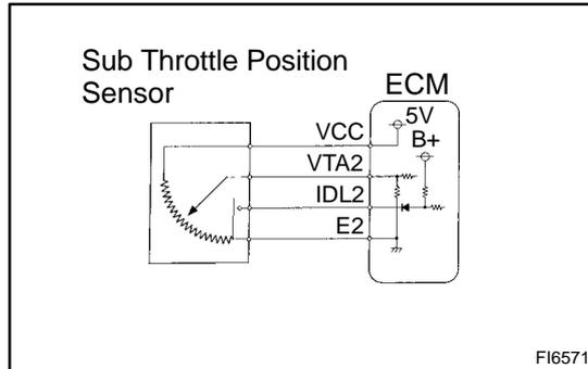
The sub throttle position sensor is built and operates in the same way as the main throttle position sensor. This sensor is used for traction control. The sub throttle valve is opened and closed by the sub throttle actuator according to signals from the throttle control ECU to control the engine output.
