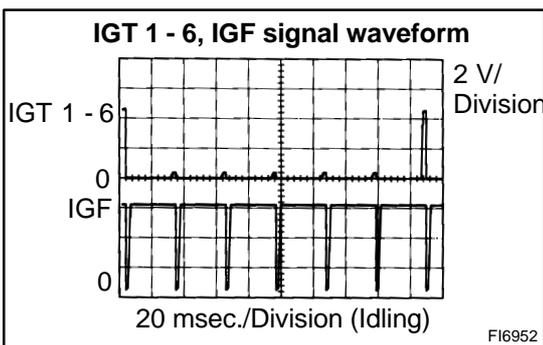
During cranking or idling, check waveforms between terminal IGT 1 - 6, IGF and E1 of ECM.
