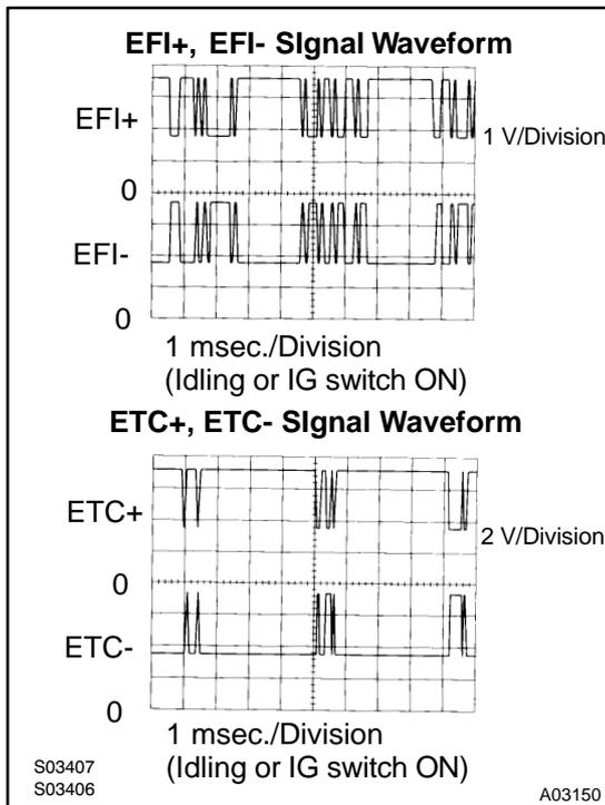
**Reference INSPECTION USING OSCILLOSCOPE**
