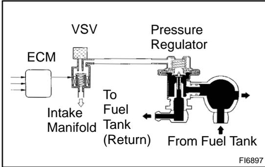
The ECM turns on a VSV (Vacuum Switching Valve) to draw the air into the diaphragm chamber of the pressure regulator if it detects that the temperature of the engine coolant is too high during engine starting. The air drawn into the chamber increases the fuel pressure to prevent fuel vapor lock at high engine temperature in order to help the engine start when it is warm. Fuel pressure control ends approx. 120 sec. after the engine is started.
