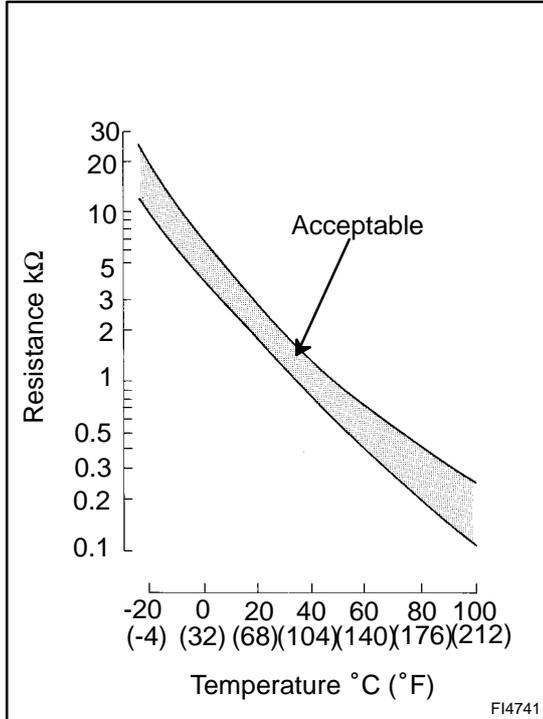
The intake air temperature sensor is built into the air flow meter and senses the intake air temperature.
