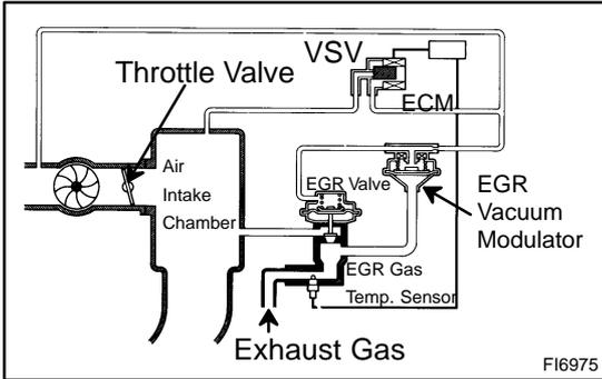
If even one of the following conditions is fulfilled, the VSV is turned ON by a signal from the ECM. This results in atmospheric air acting on the EGR valve, closing the EGR valve and shutting off the exhaust gas (EGR cut-off).
